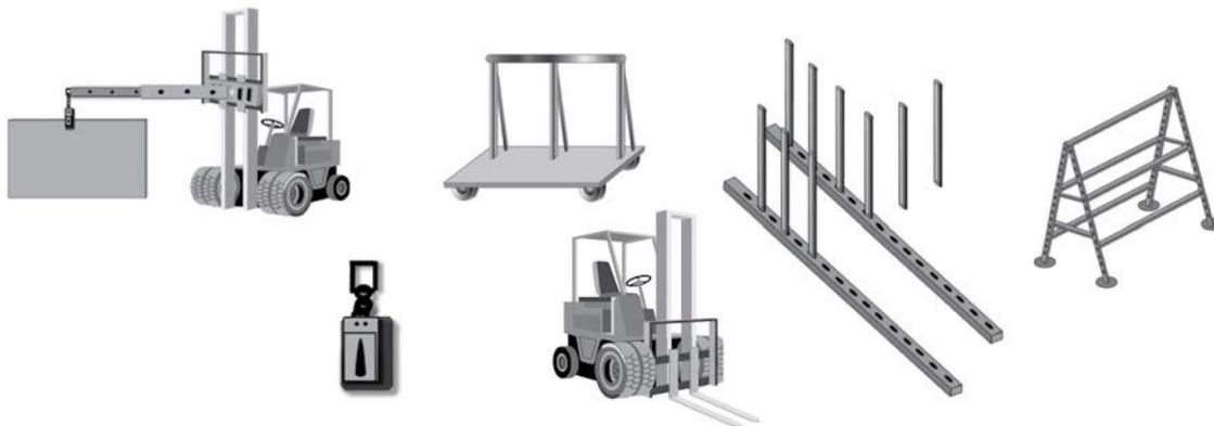
Forklifts, lifting boom, overhead cranes, jib cranes, vacuum lifter, slab clamp, A-frames, slab storage racks, A-frame carts, slab dolly, vacuum cups, fabrication tables and work benches, and racks for finished goods.
