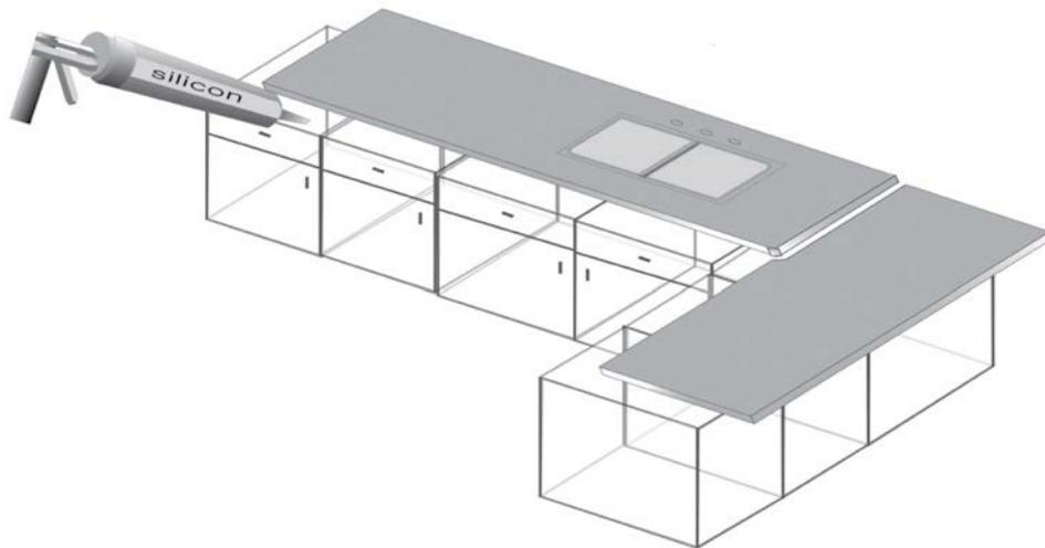
If a perimeter support system was used, place a continuous bead of clear silicone under the overhang of the top where it meets the top of the cabinet.
